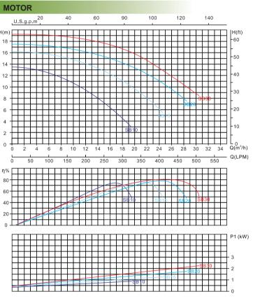
Flow curve info based on 380V/50Hz 220V/50Hz motor
