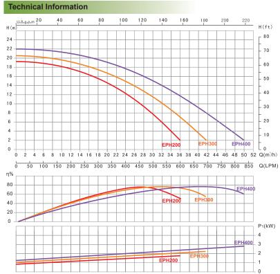
Remarks: Flow curve information based on 220V/50Hz motor.
