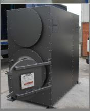
Model I8M-60—250kgs capacity—0.57m₃ capacity - 60kgs/hour burn rate
