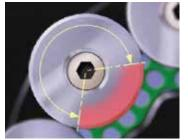
When the Disc-Blades are used, only 30 per cent of their circumferences come into contact with the woody material, hence the blades can be turned to the next sharp section when the edge has worn. This allows the blades to be turned twice before they need to be re-sharpened, in essence giving you three blades in one.
