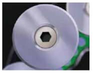
By loosening the retaining bolt, the Disc-Blades can be rotated in either direction. If damage occurs to the blade through insertion of contaminants such as stones or nails, the damaged section can simply be positioned away from the cutting area.
