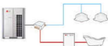
HR unit (Cooling & Hot water)
