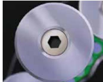
By loosening the retaining bolt, the Disc-Blades can be rotated in either direction. If damage occurs to the blade through insertion of contaminants such as stones or nails, the damaged section can simply be positioned away from the cutting area.
