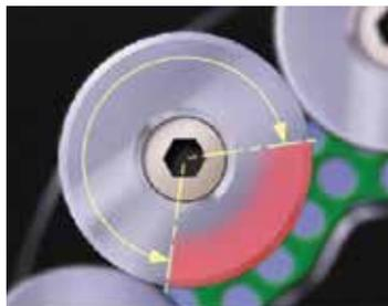
When the Disc-Blades are used, only 30 per cent of their circumferences come into contact with the woody material, hence the blades can be turned to the next sharp section when the edge has worn. This allows the blades to be turned twice before they need to be re-sharpened, in essence giving you three blades in one.
