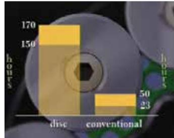
Conventional straight blades are more susceptible to damage and therefore will need to be replaced more frequently for optimal performance. When sharpened and refitted, the distance between the anvil and blade also needs to be adjusted. This does not apply to Disc-Blades, as they are sharpened from the rear so the front face does not alter and the gap remains constant.
