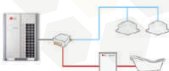
HR unit (Cooling & Hot water)
