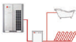
Hot water+ Radiant heating
