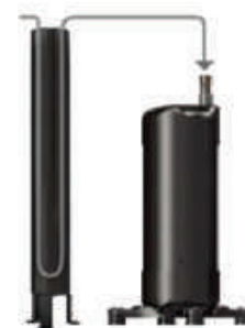
Non-receiver tank Fixed refrigerant amount
